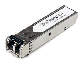
The SFP-10GBASE-LR-ST is an 10G MSA compliant fiber SFP+ transceiver that's designed, programmed and tested to work with 10GBase-LR compatible MSA switches and routers. The SFP+ transceiver module supports a maximum distance of up to 10 km (6.2 mi) and delivers dependable 10 GbE connectivity over fiber cabling.
